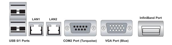
**Note:** InfiniBand ports are included on the X7DBT (6015T-INF) only. <u>To prevent damage to the port or serverboard, an InfiniBand bracket (included) must be used to secure the connector to the I/O shield.</u>
